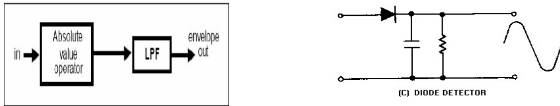
Figure 4.10: (a) Block diagram of an envelope detector (b) envelope detector.
